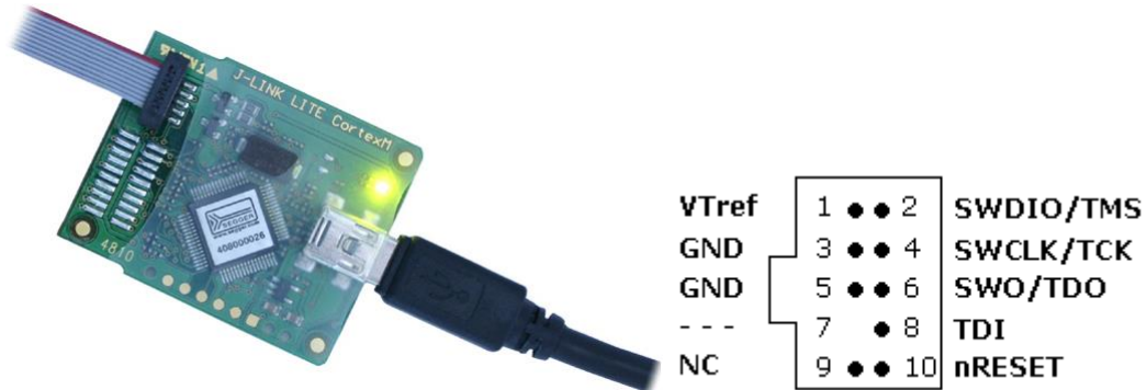
Figure 3 – SEGGER J-Link Lite Cortex-M 9-Pin JTAG with pinout (Rev 2.X+)
