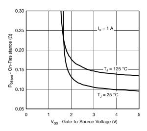
On-Resistance vs. Gate-to-Source Voltage
