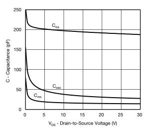
Capacitance vs. Drain-to-Source Voltage
