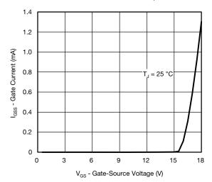
Gate Current vs. Gate-Source Voltage
