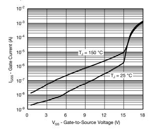
Gate Current vs. Gate-Source Voltage
