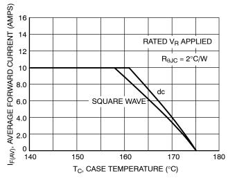
Figure 3. Current Derating, Case (Per Leg)
