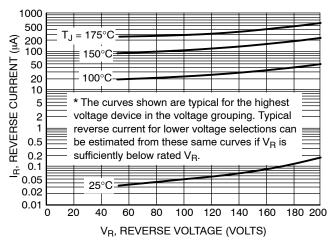
Figure 2. Typical Reverse Current\* (Per Leg)
