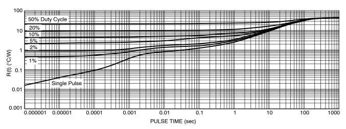
Figure 6. Thermal Response, Junction-to-Ambient
