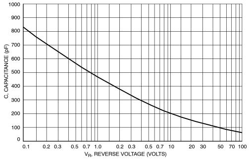
Figure 7. Typical Capacitance (Per Leg)
