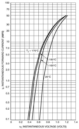
Figure 1. Typical Forward Voltage (Per Leg)
