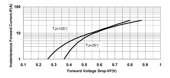
Fig.3-Typical Instantaneous Forward Voltage Characteristics
