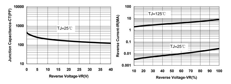
Fig.1-Typical Junction Capacitance
